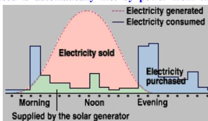
utility grid. When the home or business requires less electricity than the PV array is generating, the excess is fed (or sold) back to the utility. Used this way, the utility backs up the PV like batteries do in stand-alone systems. At the end of the month, a credit for electricity sold gets deducted from charges for electricity purchased."
